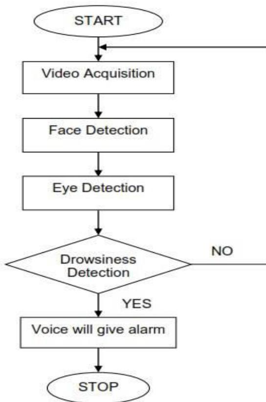
**Fig-1:** Flow-Chart about how system operates
